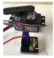
Connect the Speed controller to CH2, and the positive (+) terminal to empty CH.
