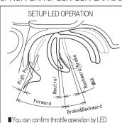
•Power on. Be careful to turn on transmitter prior to turning on ESC. (When turning off, turn off ESC prior to turning off transmitter.)
